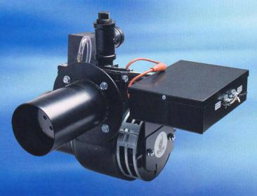
Special features: Higher static pressure than standard power gas burners. Good combustion in poor draft situations. Converts easily to fire Natural or LP Gas. Flame retention head to allow flame shapes to fit various combustion chambers. Partial premix head design to provide excellent combustion characteristics (9 to 11% CO<sub>2</sub> on Natural Gas). Industry proven controls and components.
